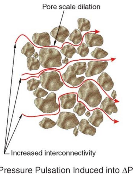
Fig. 2—Pore scale dilation increases interconnectivity in the formation.
