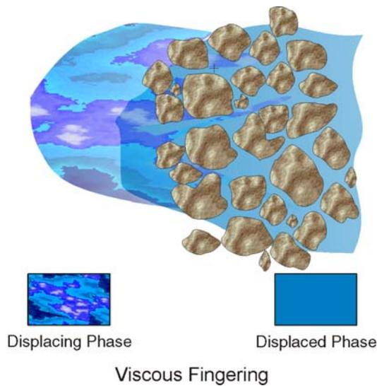
Fig. 3—An increase in the porosity and permeability of the formation results in viscous fingering.
