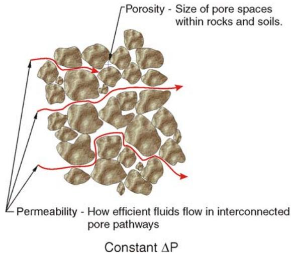
Fig. 1—The porosity of rock and soil determines how well fluids will travel through the formation.
