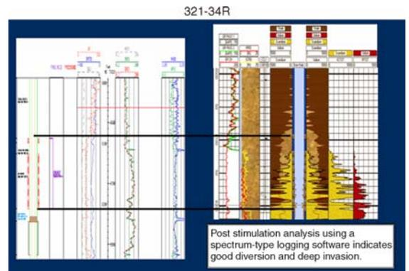
Fig. 13—Well 2 spectrum-type logging software analysis.
