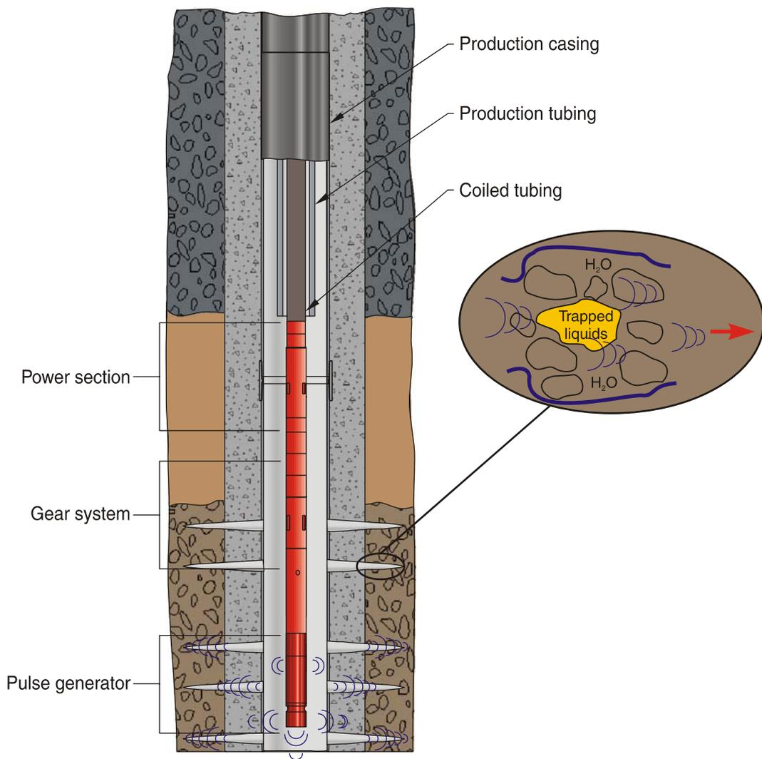
Fig. 4—The PPT stimulation tool uses downhole pulsing to dilate pores and increase porosity deeper into the formation.
