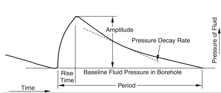
Fig. 6—Experience has shown that pore dilation and fluid movement can be best accomplished with a pressure wave as shown in the top idealized wave form.
