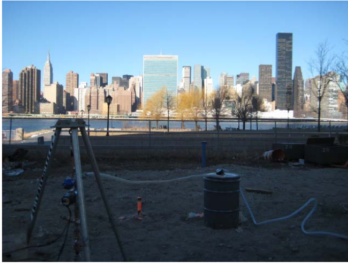
Figure 4: Wavefront Sidewinder Tool ( foreground ); Proximity of Site to the Tidally Influenced River ( background )
