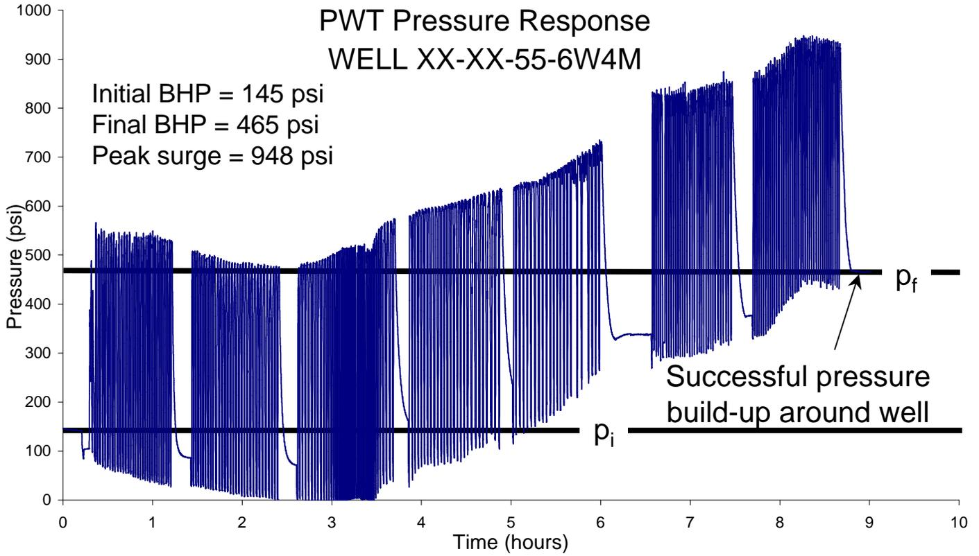
Figure 6: Pressure response and energy, a case of good response
