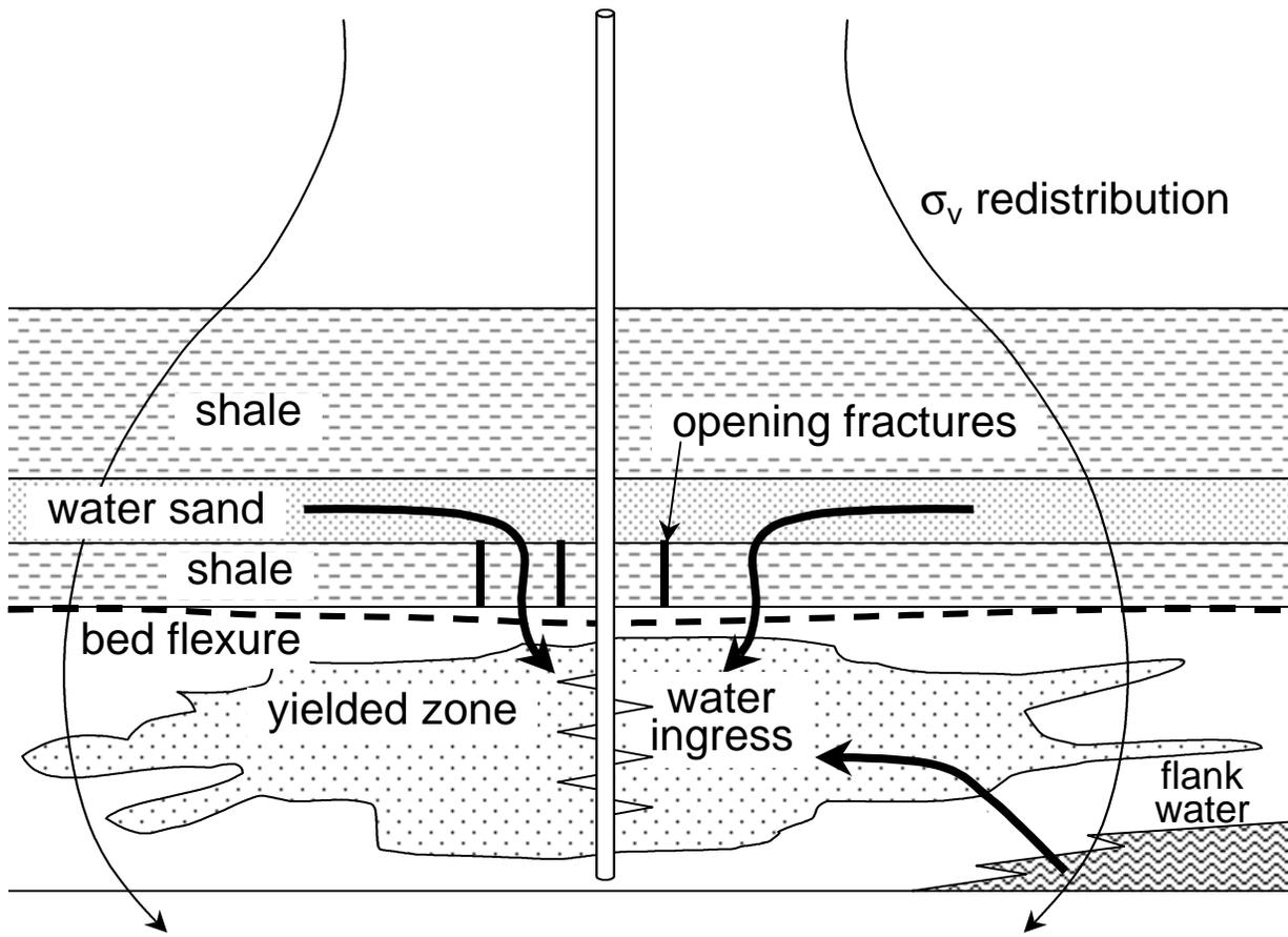
Fig 4: Water breakthrough mechanisms in CHOP wells
