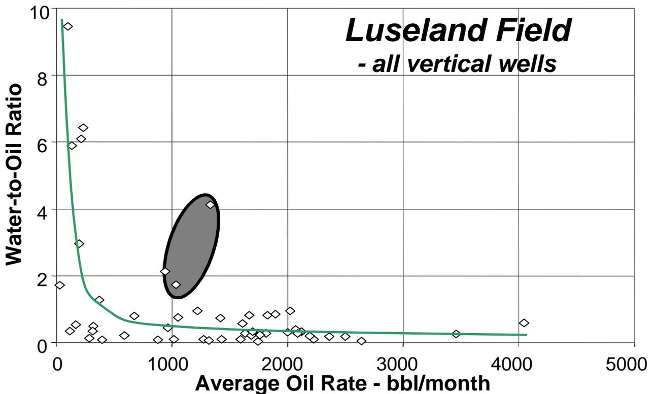
Fig 3: Normalized well behavior for the Luseland Field (Sask)
