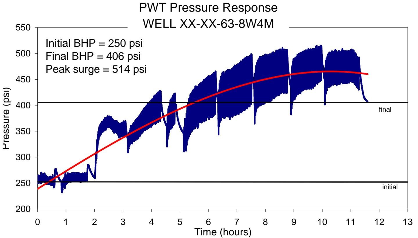
Figure 7: Pressure response and energy, a case of good pressure response despite poor energy transfer
