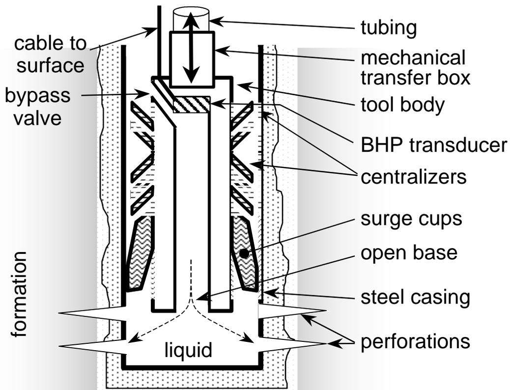
Fig 5: The basic elements of a down-hole pressure pulse device
