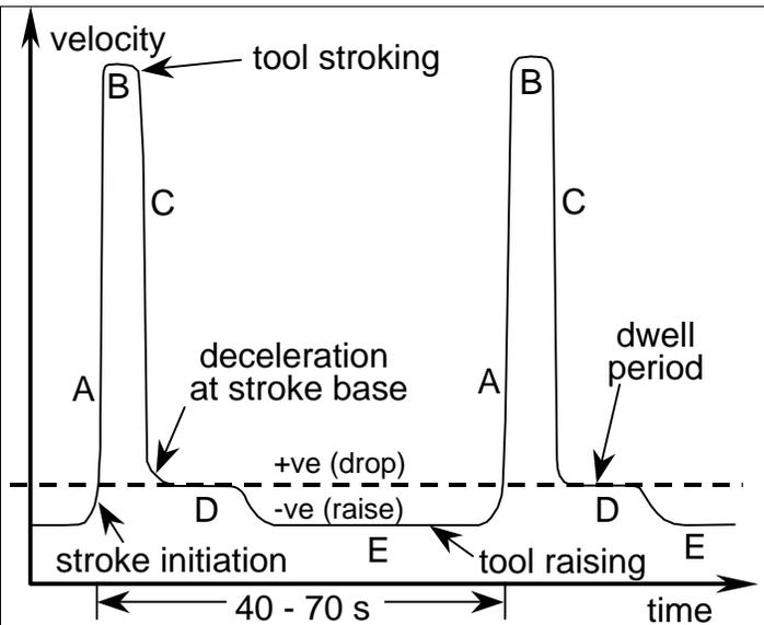
**Fig 8: Velocity vs time for PWT cycles**
