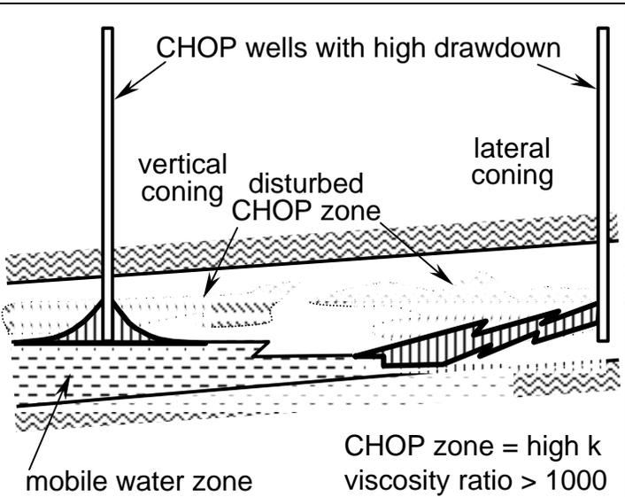
**Fig 4: Water breakthrough in CHOP wells**
