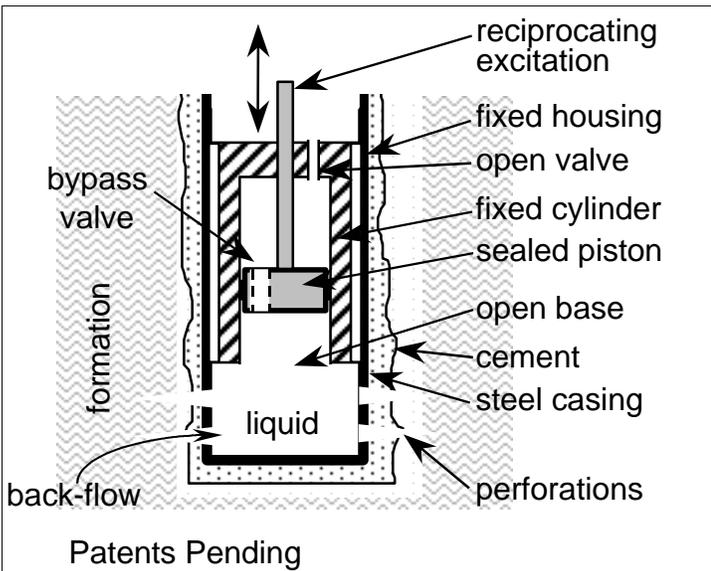
**Fig 7: Basic principle for the PWT tool**
