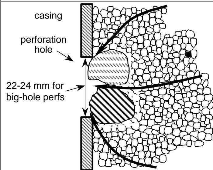
**Fig 3: Cement or concretionary fragments**
