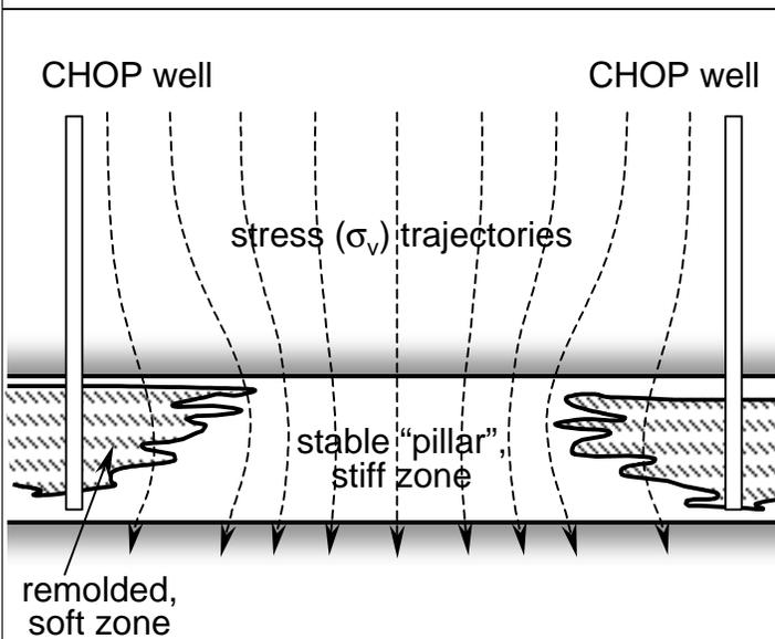
**Fig 5: Stress arching, supporting overburden**
