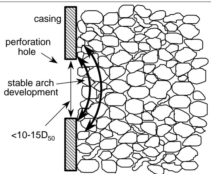
**Fig 2: Stable sand arch behind perforations**
