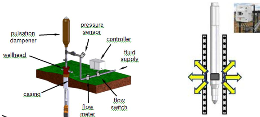
**Figure 5:** Electrical Tool Above Ground Equipment
