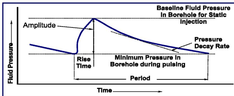
**Figure 4:** Characteristics of a Powerwave Pulse Waveform
