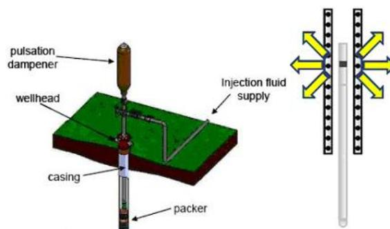
**Figure 6:** Mechanical Tool Above Ground Equipment
