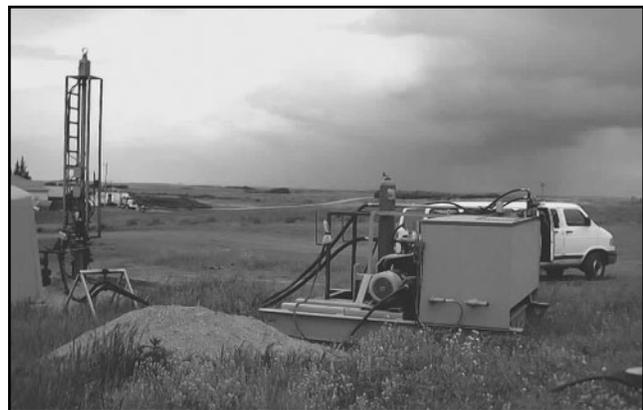
FIGURE 5: Current well head assembly pulse tool (2002).
