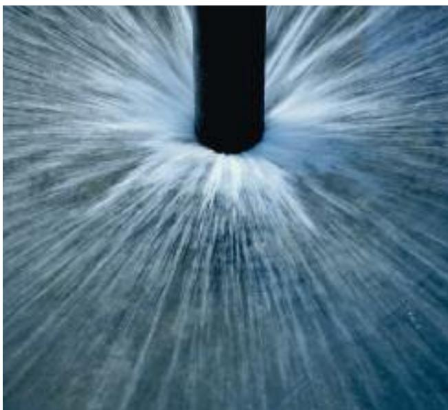
***The pulses add acceleration and momentum to the injected fluid, forcing it into the reservoirs' nooks and crannies and more impermeable rock at speeds of up to 100 metres per second***
