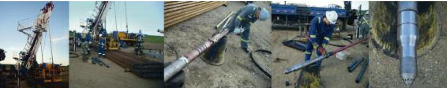
*Powerwave's down-hole tool works with conventional surface equipment, and is installed into injection wells to transform the normally steady rate of injection to a pulsating injection stream with typically 20 to 40 pulses per minute (photos: Wavefront)*
